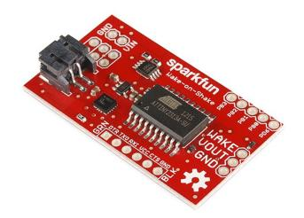
The Wake-on-Shake is intended to allow you to design a project which will remain inert for long periods of time (possibly up to several years, depending on the battery type used to power the project) until someone bumps, touches, or moves it. Its extremely low power consumption (<2uA @ 3.7V) means that, in most cases, aging related self-discharge of the battery is the limiting factor of the deployed lifespan.
