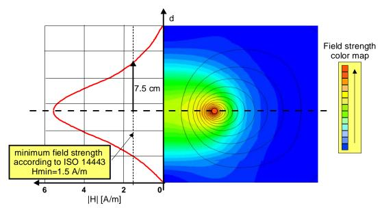
Figure 11: Non disturbed field distribution of a circular antenna
