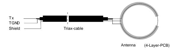
Figure 9: Electrical shielding for a 50  $\Omega$  matched antenna using a triax cable.
