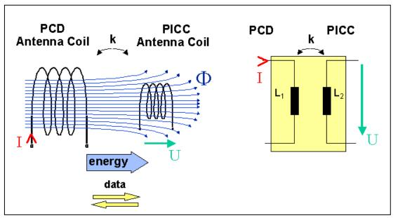
Figure 2: Transformer Model
