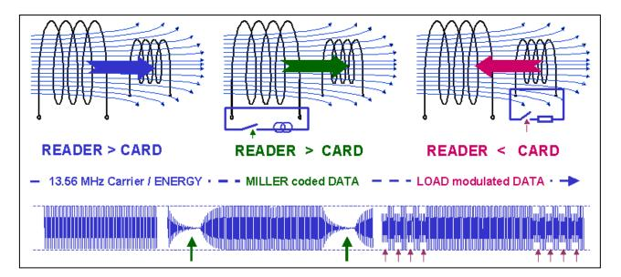
Figure 1: Mifare Interface Principle
