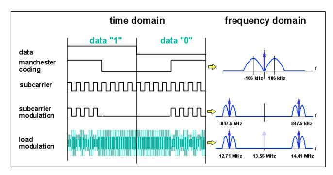
Figure 6: Principle of Data Coding PICC  $\rightarrow$  PCD, Time and Frequency Domain
