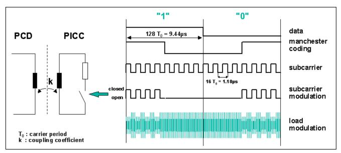
Figure 5: Subcarrier Load Modulation Principle
