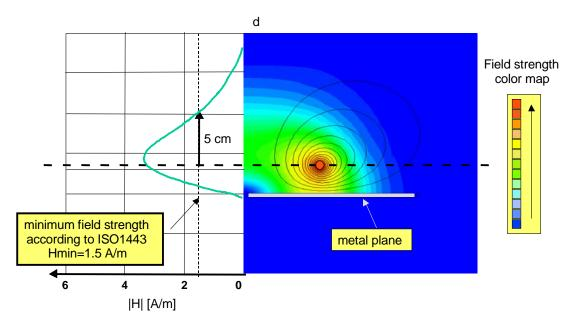
Figure 12: Field distribution of a circular antenna with a metal plane
