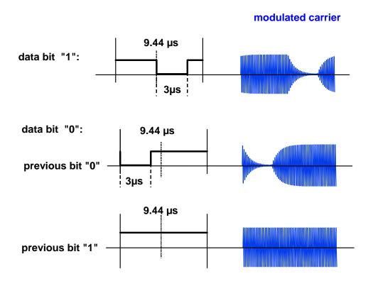
Figure 4: Data Transmission PCD → PICC, Miller Coding
