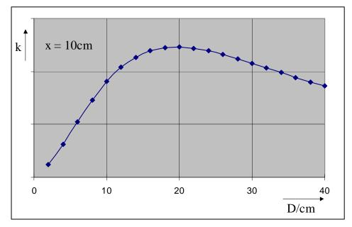
Figure 7: Coupling factor vs. Antenna diameter
