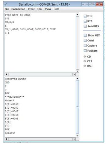
Note: The 'b' command was to verify the mode currently being programmed.
