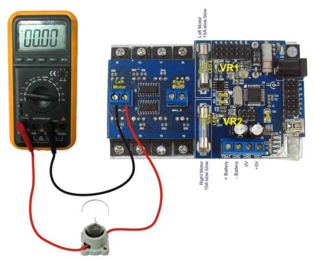
Connect the controller to a battery or DC supply by the battery terminals. Connect to your computer with the USB cable. Load and run the "Wild\_Thumper\_Diagnostic.pde" program. Click on the "Serial Monitor" icon and set the baud rate to 9600. You will see the load being measured by the processor. If you remove the fuses then you will see the current readings jump above 700. This is the highest possible reading.
