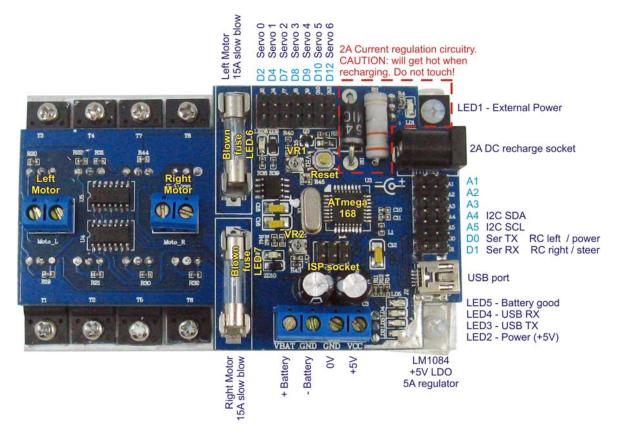
The Wild Thumper robot controller is an AVR / Arduino compatible controller that offers enthusiast the ability to get their robot up and running quickly an easily. Although relatively small in size this controller is packed with features:
