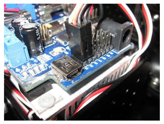
If you battery voltage gets too low (approximately 6V) then the controller will shut down to prevent malfunction and the battery charging circuit will turn on. With a DC voltage of 3-6V higher than your battery nominal voltage applied to the recharge socket your battery will begin charging until the voltage levels out for more than 5 minutes or peaks (delta V) at this point the charger will change to a trickle mode until external power is disconnected.
