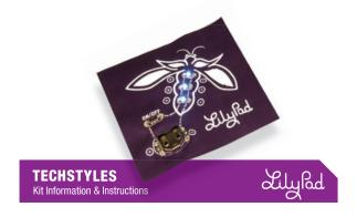
The LilyPad TechStyles kit is a great way to get started with e-textile clothing. This kit guides you through the process of using conductive thread and LilyPad LEDs to create an electronic work of art. When you're done, you'll have a greater understanding of the basic skills needed to create your own e-textiles
