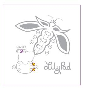
See Continue the stitch to the end. The holes should be connected by the thread, but only under the fabric.
