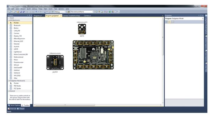
As indicated by the instructions in the text box on the canvas, the .NET Gadgeteer Designer will graphically connect all the modules for you. Right click on the design surface and select Connect all modules. You can move the modules around on the design surface to make the connections easier to read. You can also delete any connection by right clicking on the connection and selecting Delete. Make sure both modules are connected as in the diagram below.
