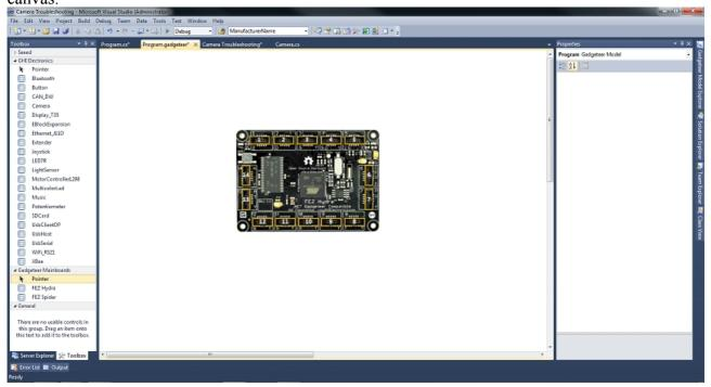
If you want to use a different mainboard, open the toolbox, and drag the mainboard icon of your choice onto the designer surface. The following illustration shows the open toolbox with two mainboard options.
