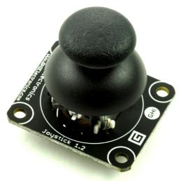
Turn the **Joystick** module over. Next to the connector is the letter **A**. This means that a **Joystick** module can be connected to one of the sockets labeled **A** on a mainboard.
