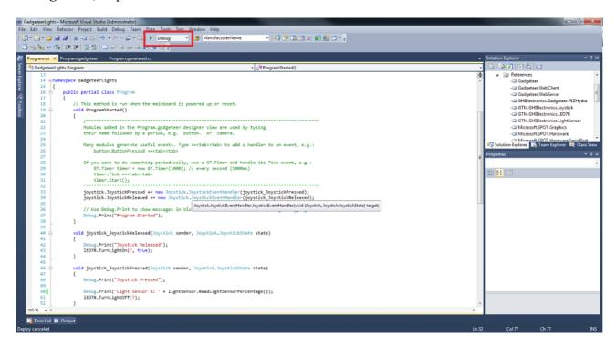
Make sure that the **Output Window** is visible by pressing the **CTRL** + **ALT** + **O** key combination on your keyboard. If you have enabled sounds, you should hear Windows make the "USB disconnected" sound, followed by the "USB connected" sound as the Mainboard reboots. The **Output Window** should show the process of loading various files and assemblies. The final line, which appears once the application begins to run, should read **Program Started**.
