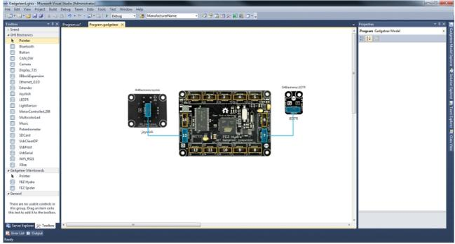
To manually set a connection, click on a socket in the diagram and hold down the left mouse button. Then you can drag a line that represents the connection from a module socket to a mainboard socket or in the opposite direction from the mainboard to a module. The sockets that the module can use will light up in green, as shown in the following illustration.
