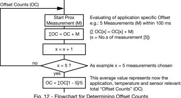
Fig. 12 - Flowchart for Determining Offset Counts
