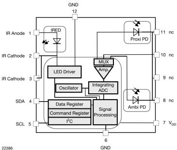
Fig. 2 - VCNL4000 Detailed Block Diagram
