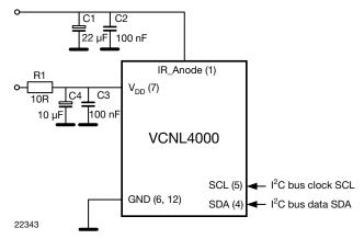
Fig. 4 - VCNL4000 Application Circuit
