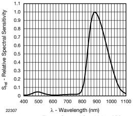
Fig. 9 - Spectral Sensitivity of PD
