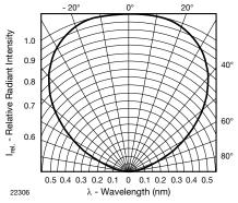
Fig. 5 - Angle of Half Intensity of the Emitter
