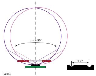
Fig. 7 - Emitter and Detector Angle and Distance
