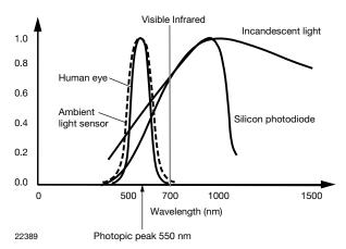
Fig. 17 - Relative Spectral Sensitivity vs. Wavelength
