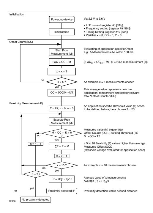
Fig. 15 - Flowchart for Proximity Sensing
