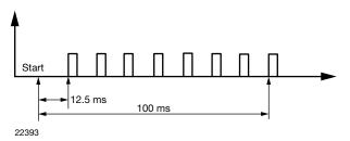
Fig. 20 - Ambient Light Measurement with Averaging = 8
